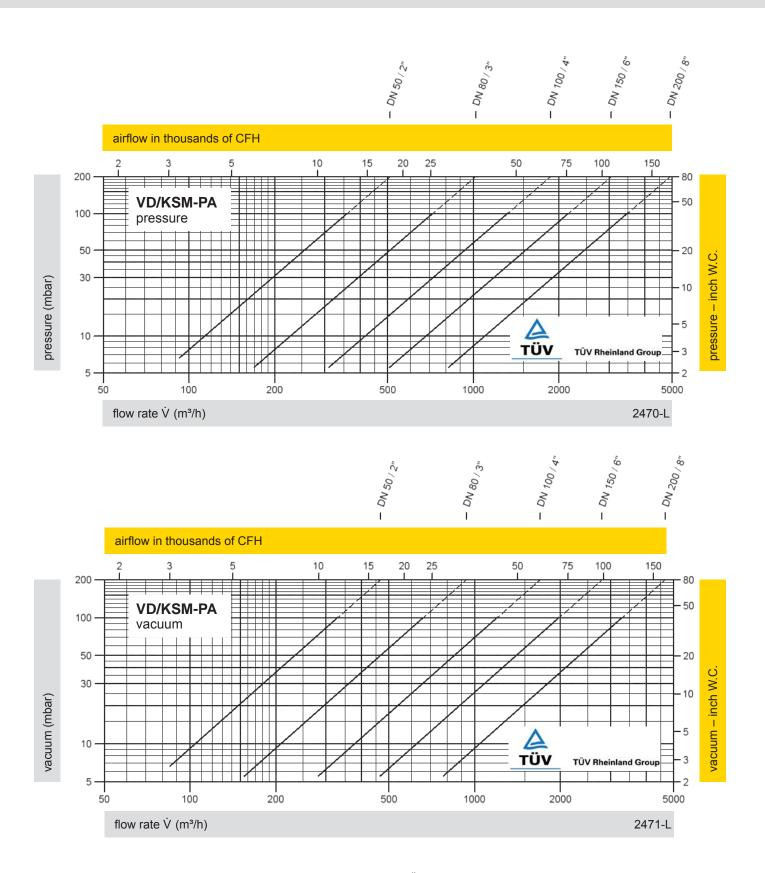
The flow capacity charts have been determined with a calibrated and TÜV certified flow capacity test rig. Volume flow  $\dot{V}$  in (m³/h) and CFH refer to the standard reference conditions of air ISO 6358 (20°C, 1bar). Conversion to other densities and temperatures refer to Vol. 1: "Technical Fundamentals".
