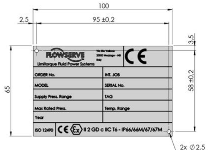
Figure 1: LPS Actuator Nameplate
