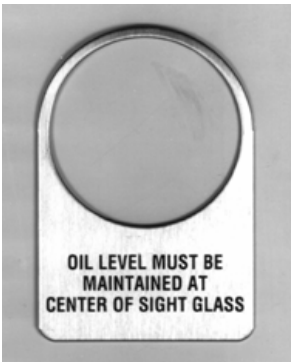
Figure 6-15 - "Oil level must be maintained at center of sight glass"
