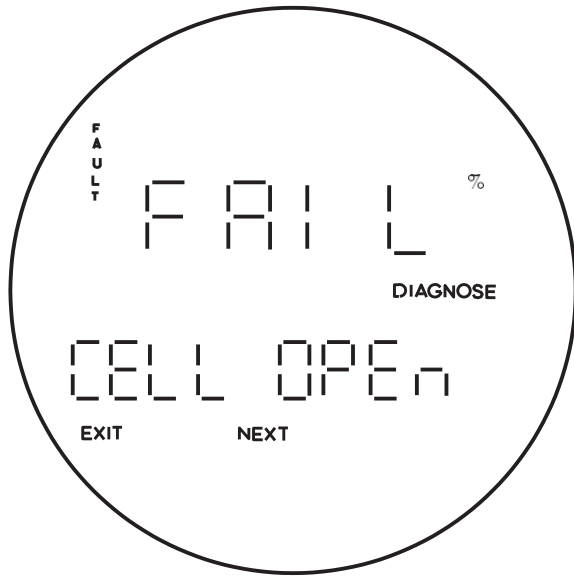
Figure 5-9. Fault 5, O2 Cell Open
