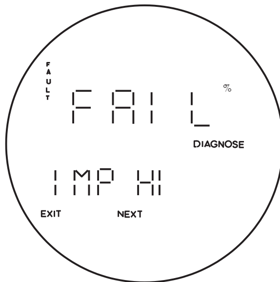
Figure 5-10. Fault 6, Cell Impedance Too High
