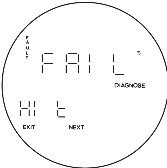
Figure 5-8. Fault 4, High Probe Temperature
