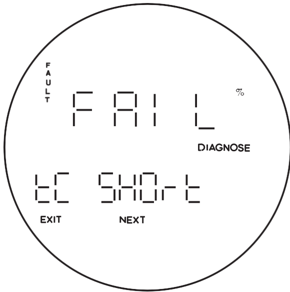
Figure 5-7. Fault 3, Shorted Thermocouple
