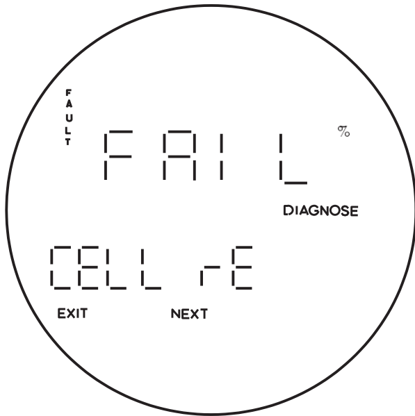
Figure 5-11. Fault 7, Reversed O 2 Cell
