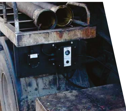
The Earth-Rite II MGV static grounding system can be mounted on vacuum trucks and tank trucks.
