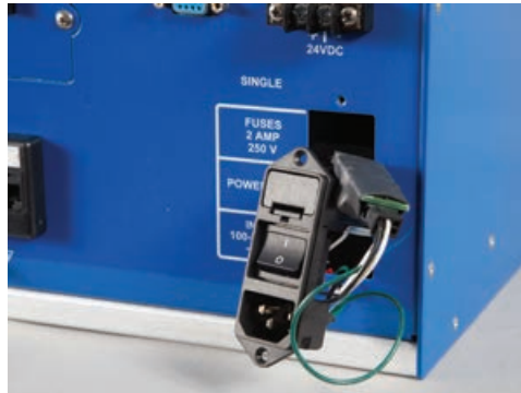
Figure 10.3 - Removing Main AC Input Power Module
