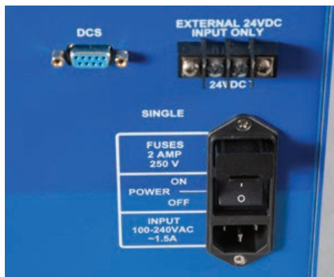
Figure 10.5 - Removing Fuse Holder
