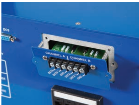
Figure 10.8 - Removing Network Surge Protector
