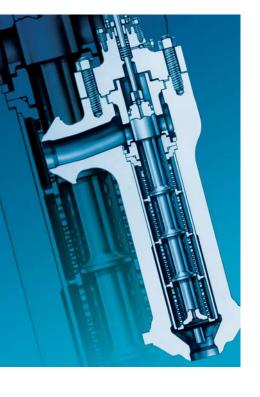
Design CAV4 control valve with Cavitrol® IV trim is designed specifically for liquid applications, such as boiler feedwater recirculation, where pressure drops are above 3000 psi and cavitation is a problem.
