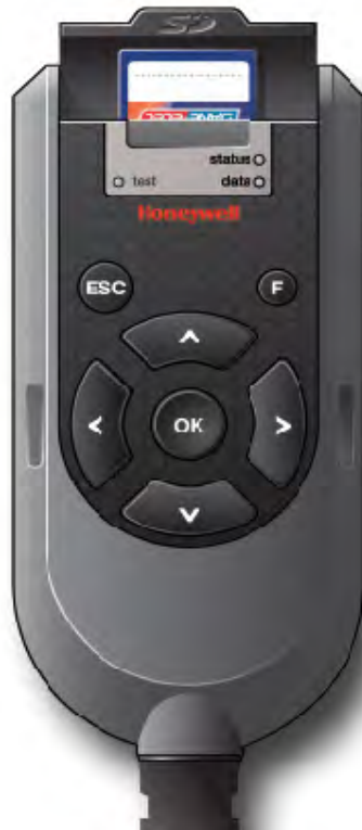
FIGURE 5-6 SD card location in LAD (lid opened)
