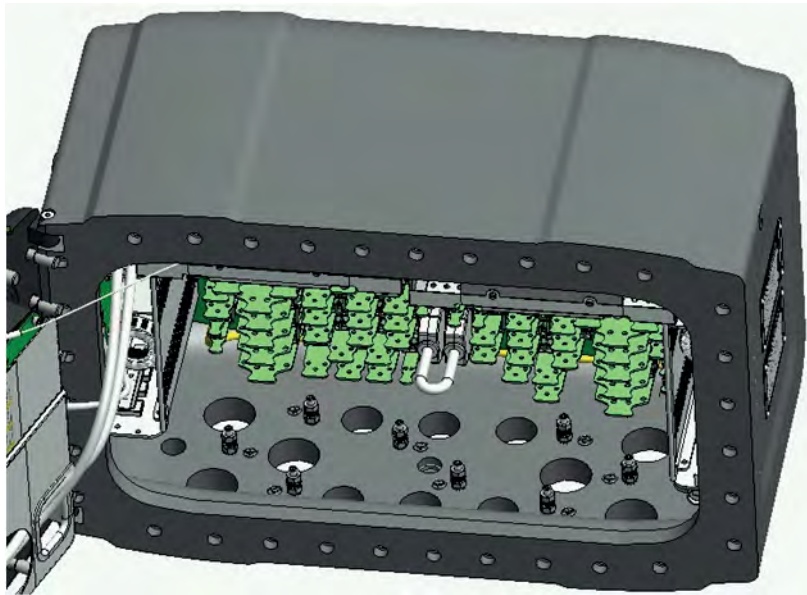
Internal grounding connections of the MSC-A
