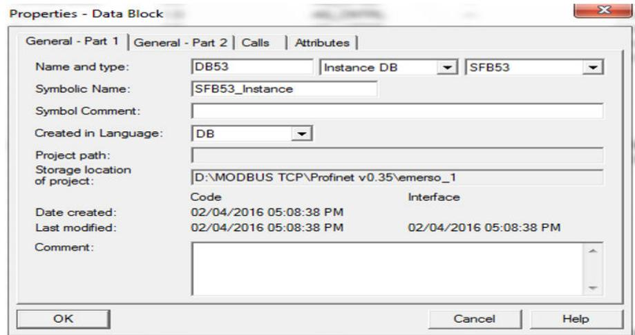
The second of the two data block DB instances is added. The SIMATIC Manager displays the entries.
