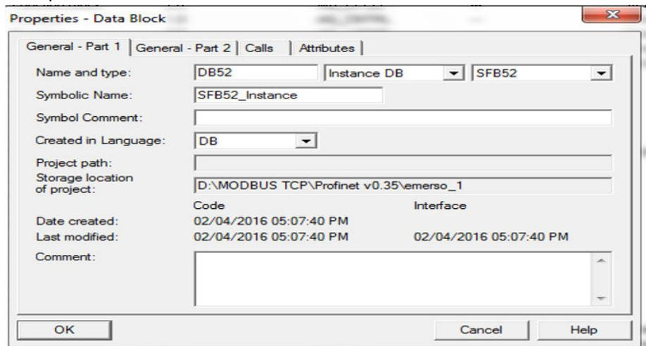
The first of the two data block DB instances is added.
