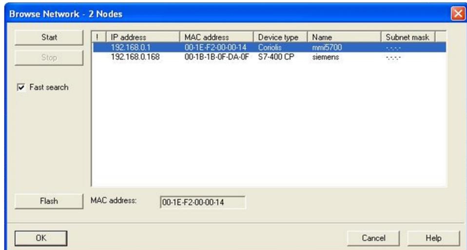
8. Choose PLC > Ethernet > Verify Device Name to verify the device name was properly assigned.
