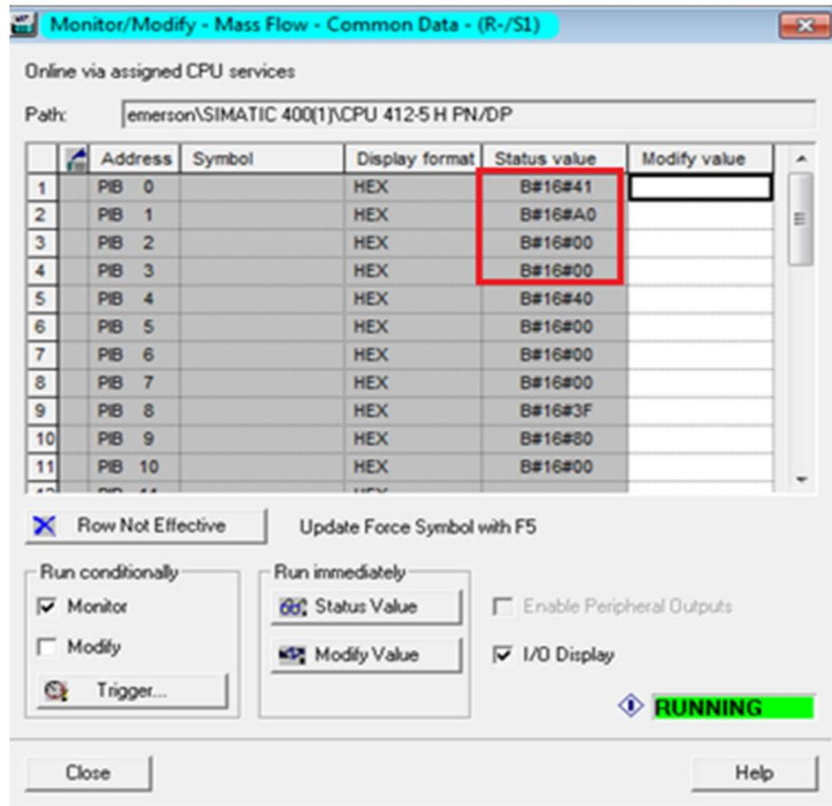
3. If the transmitter is still not communicating, from the transmitter display, choose Menu > Configuration > Ethernet settings > Primary Protocol > Profinet to verify that PROFINET is the configured primary protocol on the Model 5700 Ethernet transmitter.
