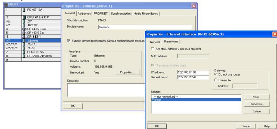
The network settings of the S7 400 PLC Ethernet interface are configured.
