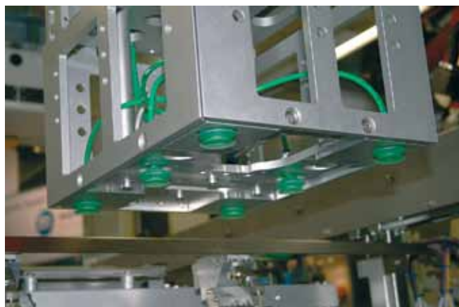
Bellows suction cups NSPB1 being used in top-loading machines
