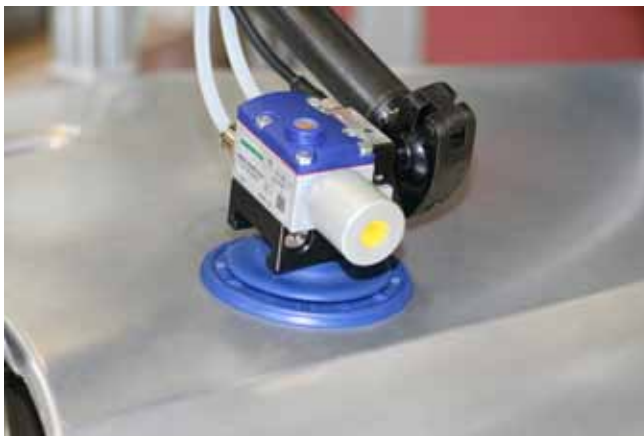
Decentralized vacuum generation by means of ejector NSEAC-RP with blow off system right on suction cup
