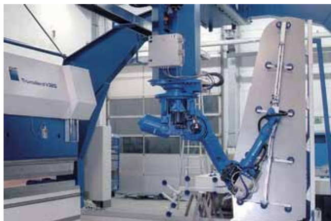
Flat suction cups NSAFX being used for handling sheet metal parts
