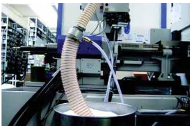
Vacuum generation by means of feed ejector NSEC for transporting granulates
