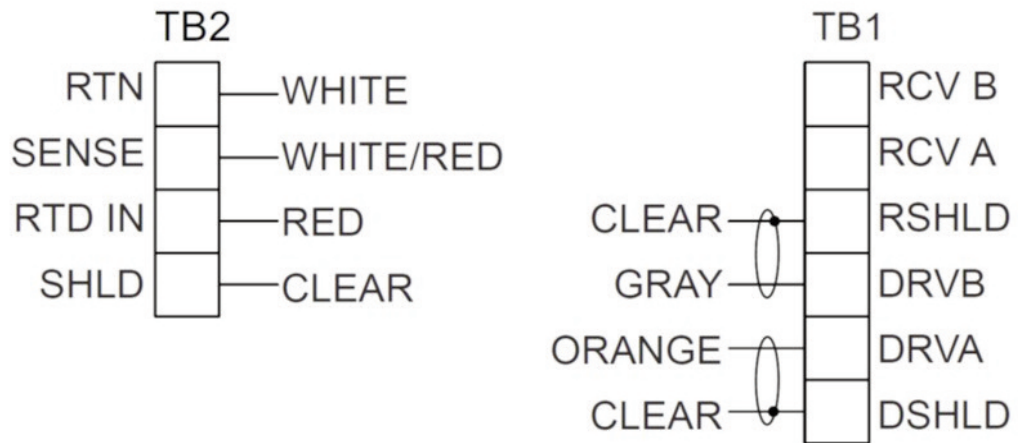
Figure 3-4: Wiring for Rosemount 56 and 1056 transmitters
