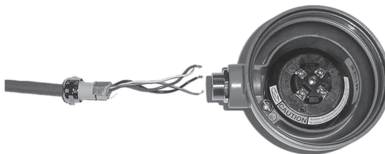
Figure 3-9: Installing the gland body
