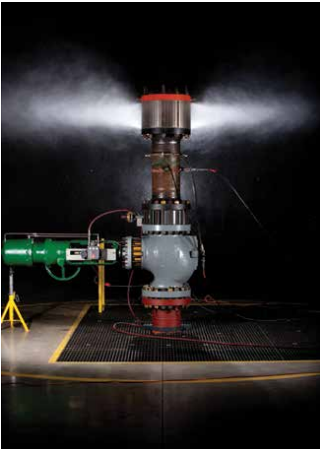
Test programs are conducted on Fisher control valves, valve trim, silencers, diffusers, and spargers as well as tees, elbows, reducers, and expansions to determine their contribution to overall noise.
