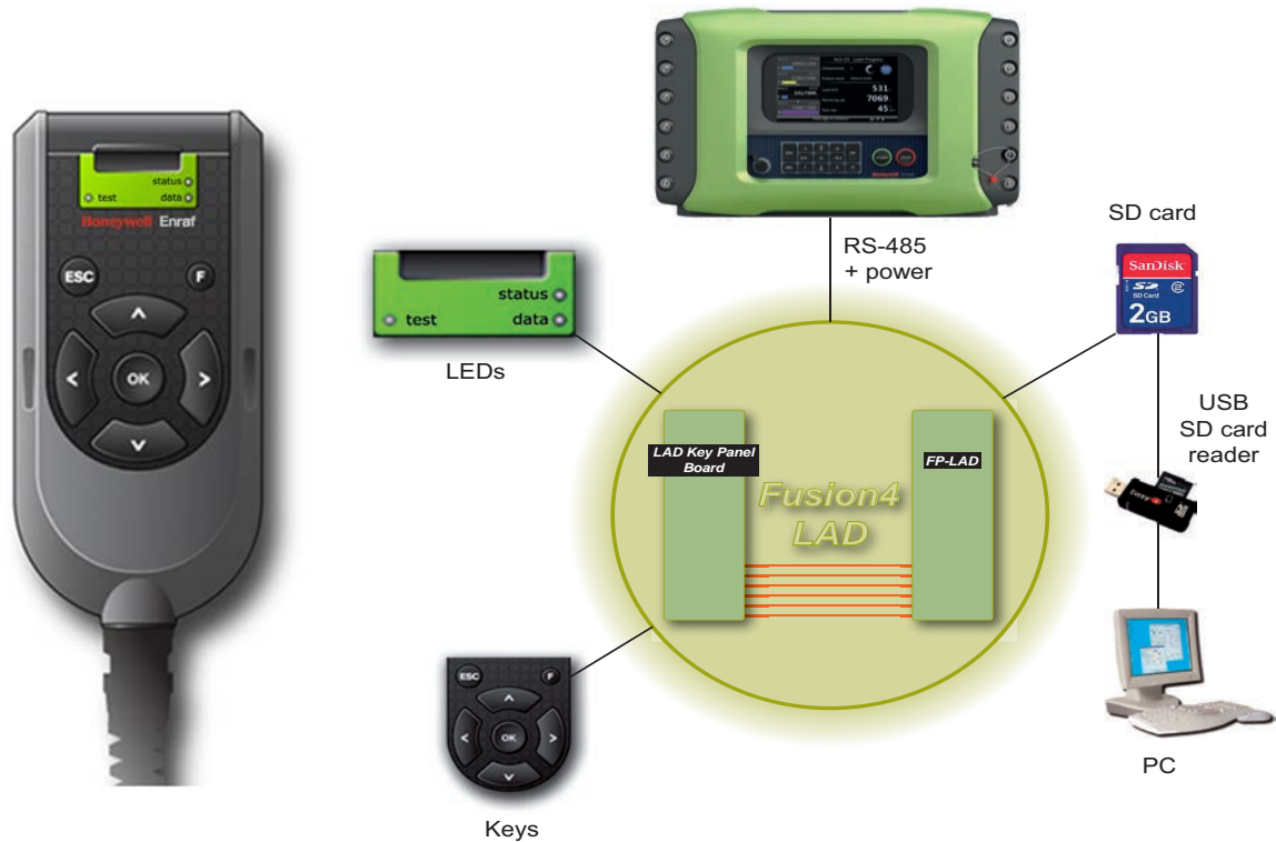
FIGURE 5-3 LAD and its system overview
