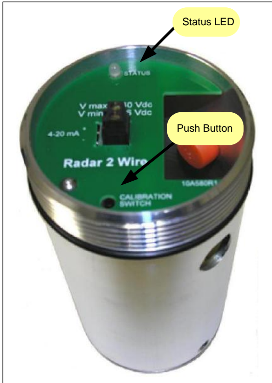
Figure 29. The illustration shows the location of the LED and the push button for both Radar and Ultrasonic sensors.
