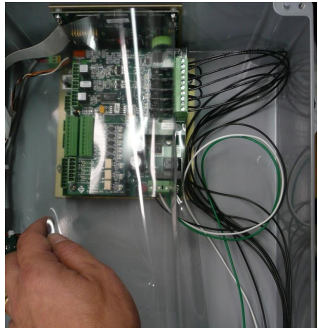
Figure 2.5 Removal of AC Wiring Side Partition
