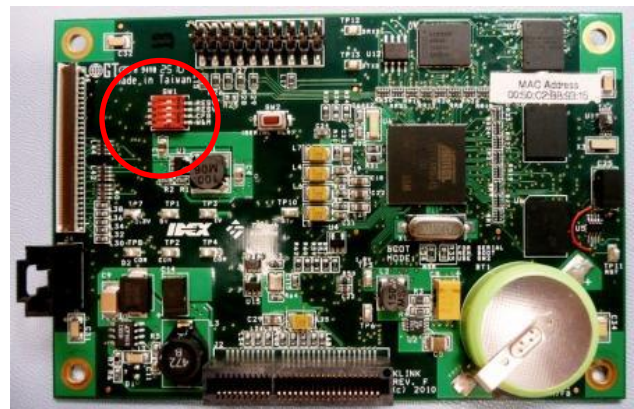
Figure 5.5 CPU DIP Switches for Program and W&M Access (rev 2.0)
