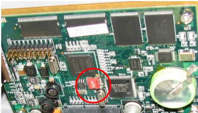
Figure 5.4 CPU DIP Switches for Program and W&M Access (rev 1.0)
