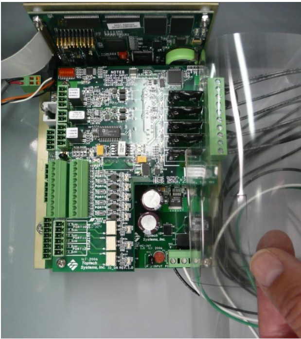
Figure 2.4 AC Supply Terminal Block Access
