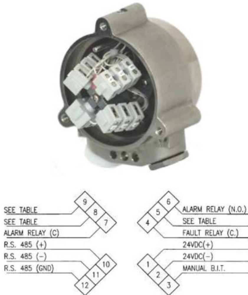
Figure B-1: Wiring terminals
