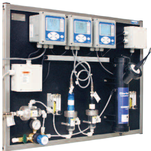
Figure 87. Multiple 1056 instruments with HART communication, shown mounted on a panel for simple Plug-N-Plumb installation. Four sensors (conductivity, pH, dissolved oxygen, and turbidity) are mounted with a flow regulator. The system shown was designed on a stand-alone panel for table-top mounting but can be purchased as a panel mount version.
