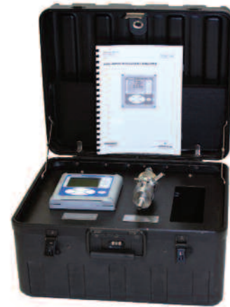
Figure 76. The 1056 conductivity instrument and 404 conductivity sensor are hard mounted into a protective case. Each unit includes all cabling and tubing needed for connection to a water system.
