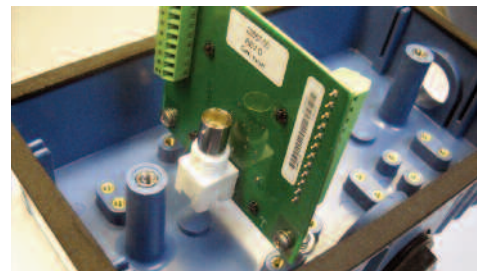
Figure 71. Junction Box PN 23555-00 is used for pH and ORP sensors only. A preamplifier board is mounted internally.
