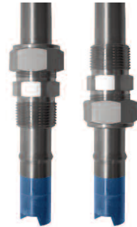
Figure 44. The 23166-00 (or -01) metal process connector, shown with the 3300HT PERpH-X sensor, allows various insertions depths, depending on where the user locates the compression fitting. Also the threads can be switched to face the top end of the sensor (right) for connection to submersion pipes.
