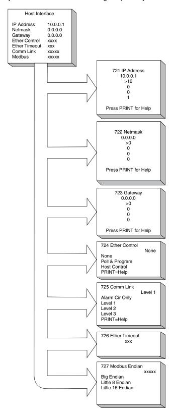
The IP, Netmask and Gateway Addresses are in the form of four numbers separated by ".". The range of each number (also known as "octet"), is 0-255. The microLoad.net screen for entering these values lists the present octet values vertically.
