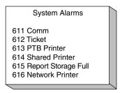
611 CM: Communications Alarm. Indicates a failure on one of the communication channels.
