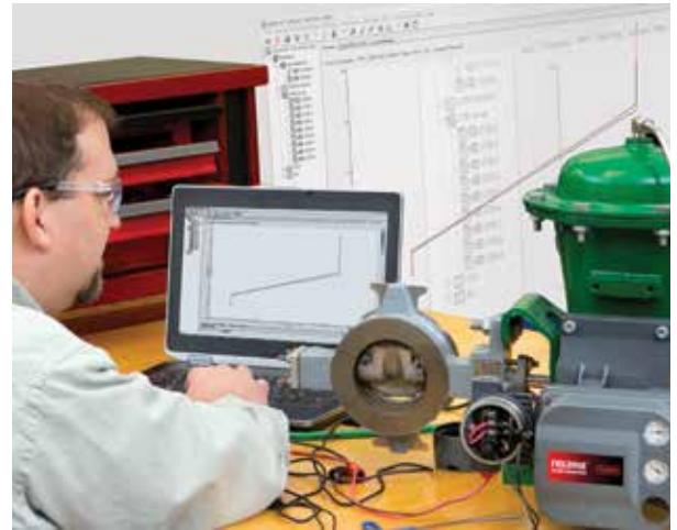
Using a valve signature series test, you can easily track the operating health of your control valve without removing it from the line.
