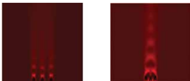
Laser shadowgraphs show jet independence from three properly spaced holes (left). The same three holes spaced too closely (right) show jet interaction, which leads to additional noise. Being able to predict and control jet interaction can reduce the noise produced by up to 40 dBA.
