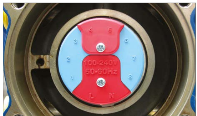
Fig 7.16 IS Terminal Block
