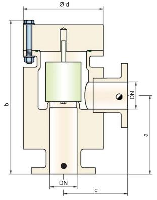
= Tank connection for pressure relief function
