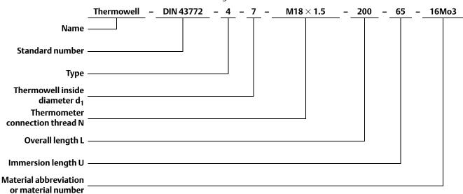
Table 10, Table 11, and Table 12 show all required thermowell dimensions necessary to conform to DIN 43772 Type 4 and the relationship to the Rosemount 114C Thermowell.
