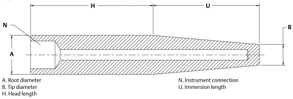
Table 15. Weld Mounted Thermowells (Weld-in)(1)
