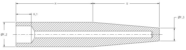
H. Head length  $\varnothing$  F\_2,  $\varnothing$  F\_3, and H\_1, refer to Table 13.
