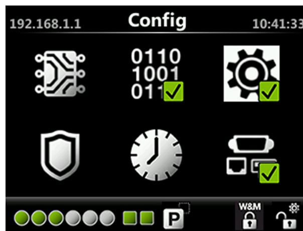
FIGURE 7-10 Status Dashboard: configuration settings are unlocked
