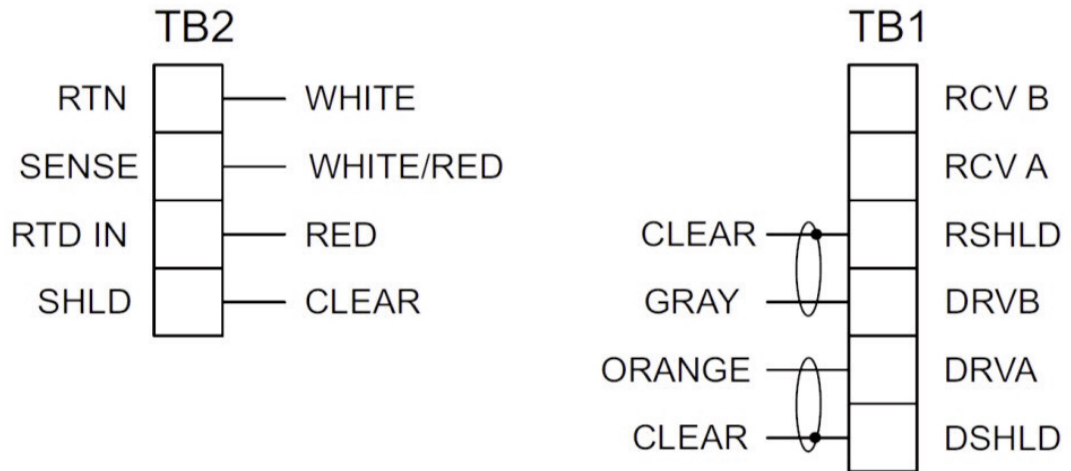
Figure 3-4: Rosemount 140/141/142 Sensor Wiring to Rosemount 1066 Transmitter
