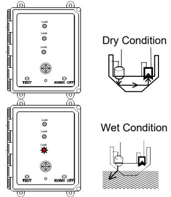
3. Since system sensors are solid state and work with normally closed loop of light, sensors can be tested as follows:
