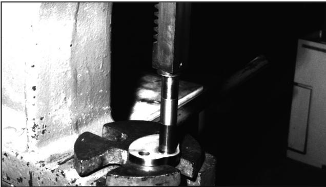
**Figure 13 – Press Shaft Out of Cam**
