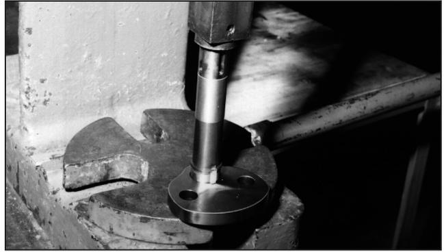
**Figure 14 – Press Shaft into Cam**
