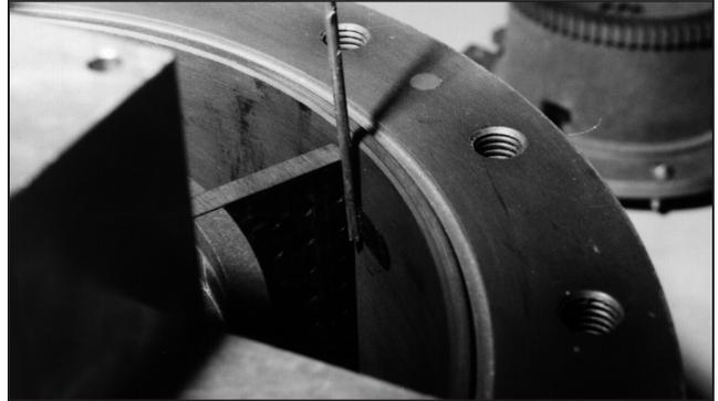
**Figure 20 – Measure Blade Tip Clearance**
