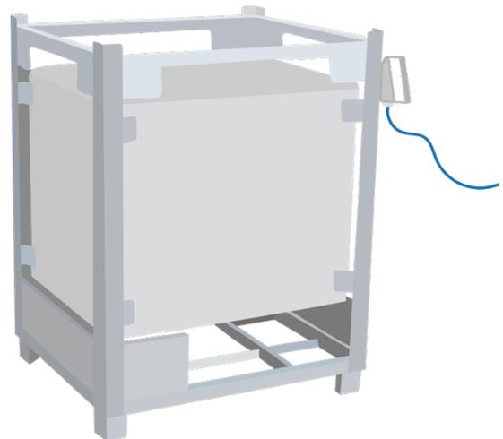
Equipment can only be grounded by ensuring a low resistance connection to verified true earth grounding points (e.g. copper bus-bars). Other equipment used in the process can be bonded to the equipment that is grounded ensuring static electricity does not accumulate on the equipment in the overall system.
