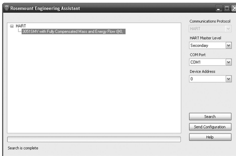
Figure 2-12: Engineering Assistant Device Connection Screen
