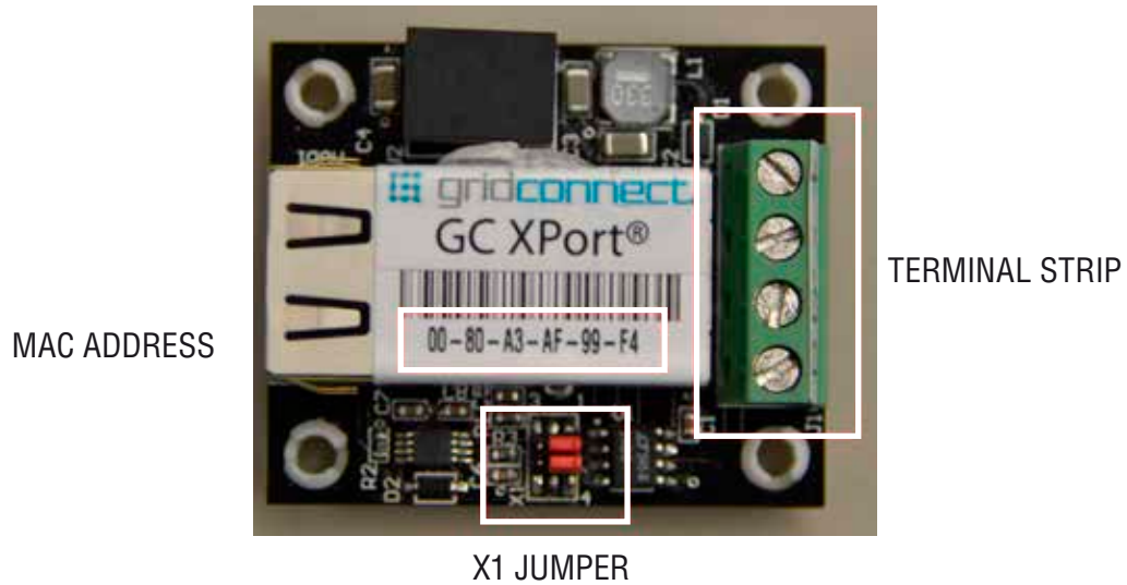
Figure 3.13 - Jumper on RS-485 to Ethernet adapter
