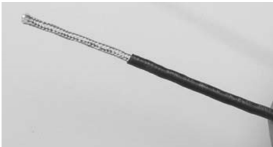
Figure 3.3 – Removing outer plastic jacket
