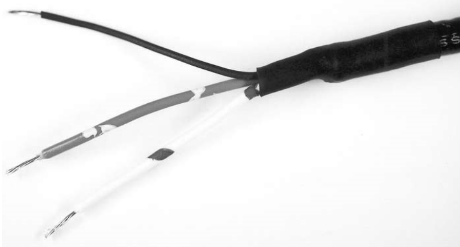
Figure 3.6 – Applying heat shrink tubing
