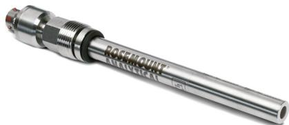
Rosemount Hx438 dissolved oxygen sensor provides a drift-free signal and maintains its calibration value for up to 50 steam sterilization cycles. It can be used in the biotechnology, pharmaceutical, chemical, and food processing industries. Rosemount Hx438 dissolved oxygen sensor uses a 4-pin connection plug for quick disconnection from the cable (sold separately).
