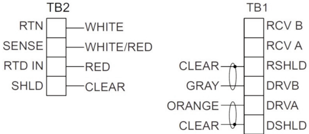
Figure 3-4: Wiring for Rosemount 56 and 1056 transmitters
