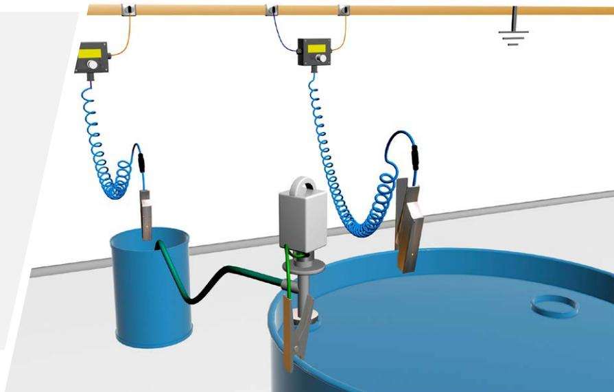
The Bond-Rite CLAMP contains a bright green LED which pulses continuously when it detects that the resistance between the equipment to be grounded and the site's verified earth ground is 10 Ohms or less.
